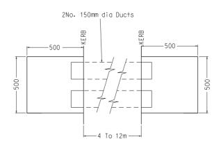
The crossing is to include laying 2No. 150mm dia ducts (provided by WPD), a 500x500mm opening in the footpath each side of the road, removing and reinstating kerb edges as necessary and complete reinstatement on completion of works.
