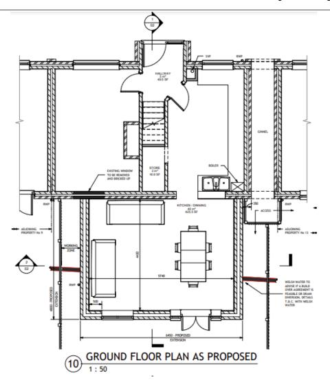
Figure 3 Proposed ground plan of rear extension
