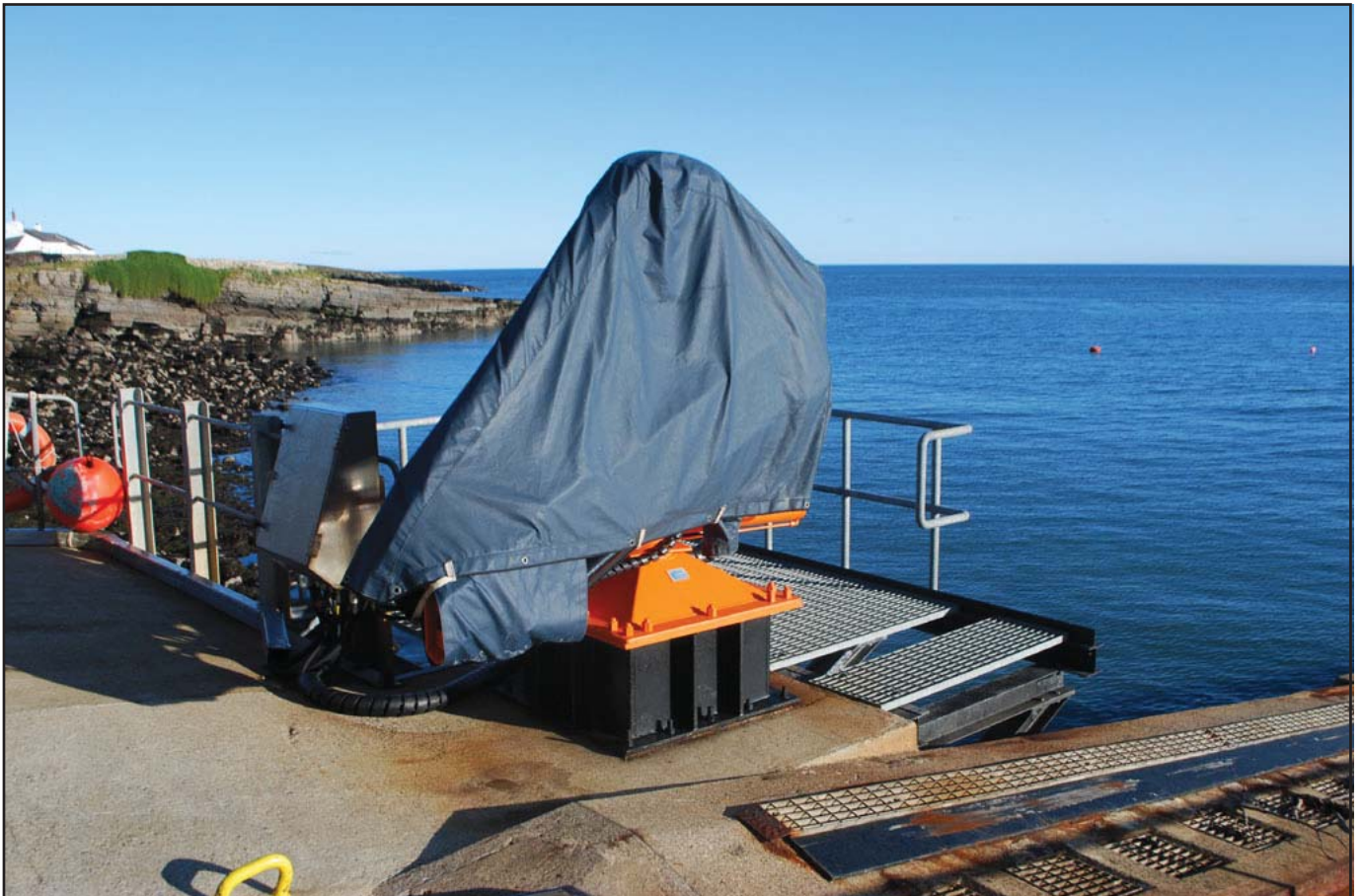
Plate 18 – Hydraulic lift to place inshore lifeboat on slipway
