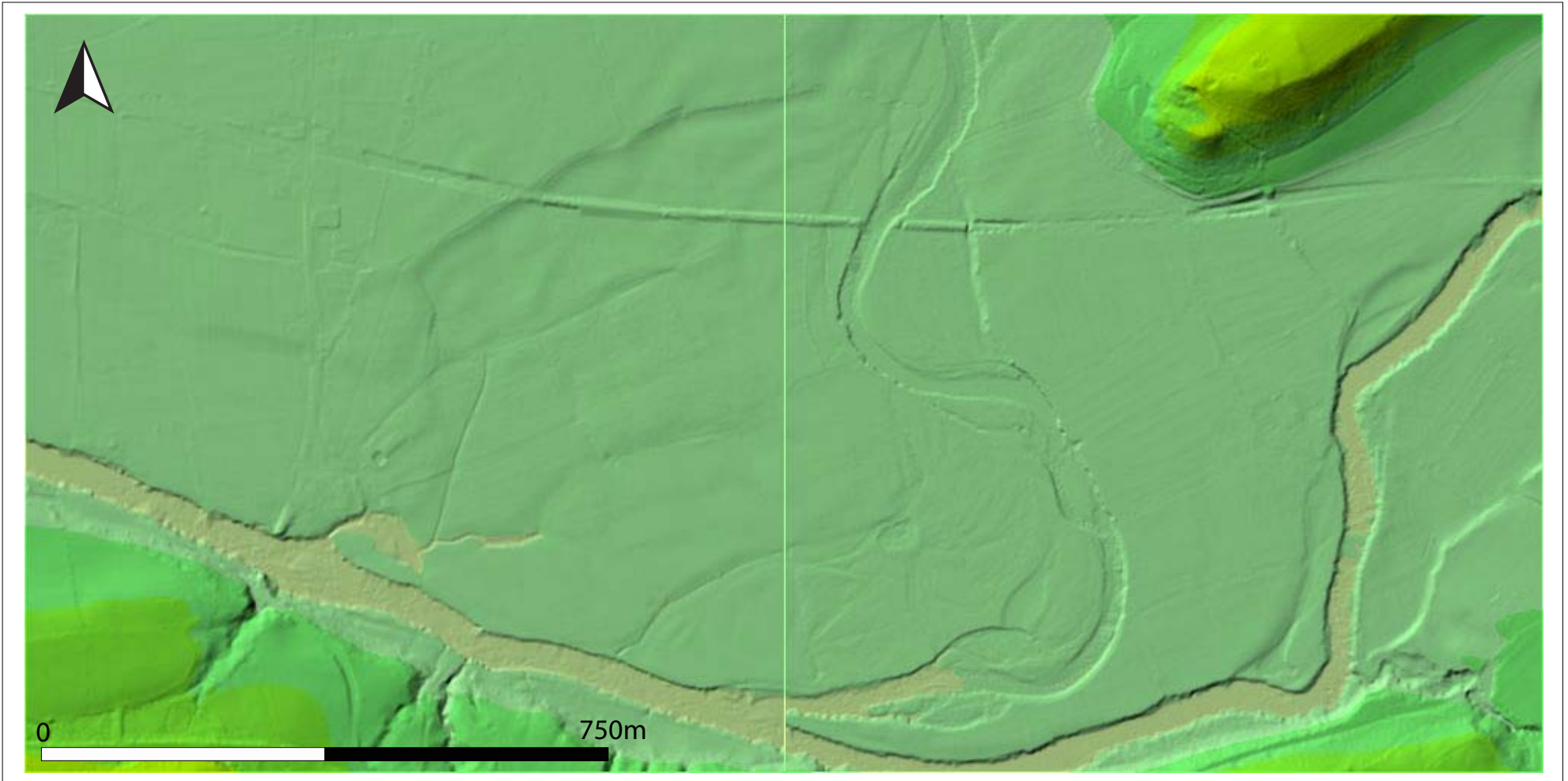
Fig 5: LiDAR data for Area A showing confluence of rivers Tywi and Cothi. Note evidence of previous courses of river Cothi across floodplain area
