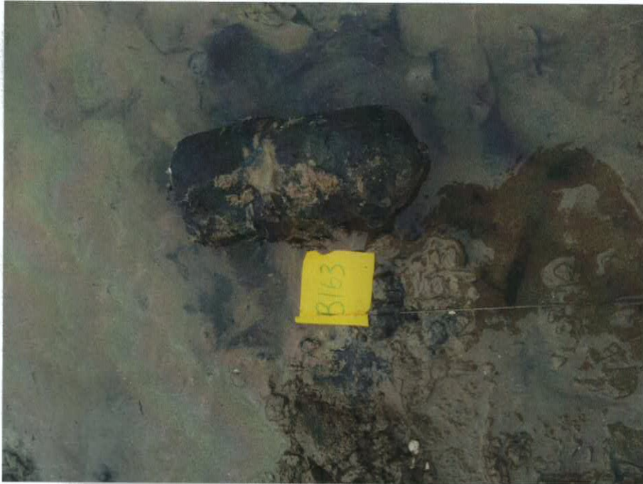
Munition – This target was found to be a 25lb Armour piercing shell
