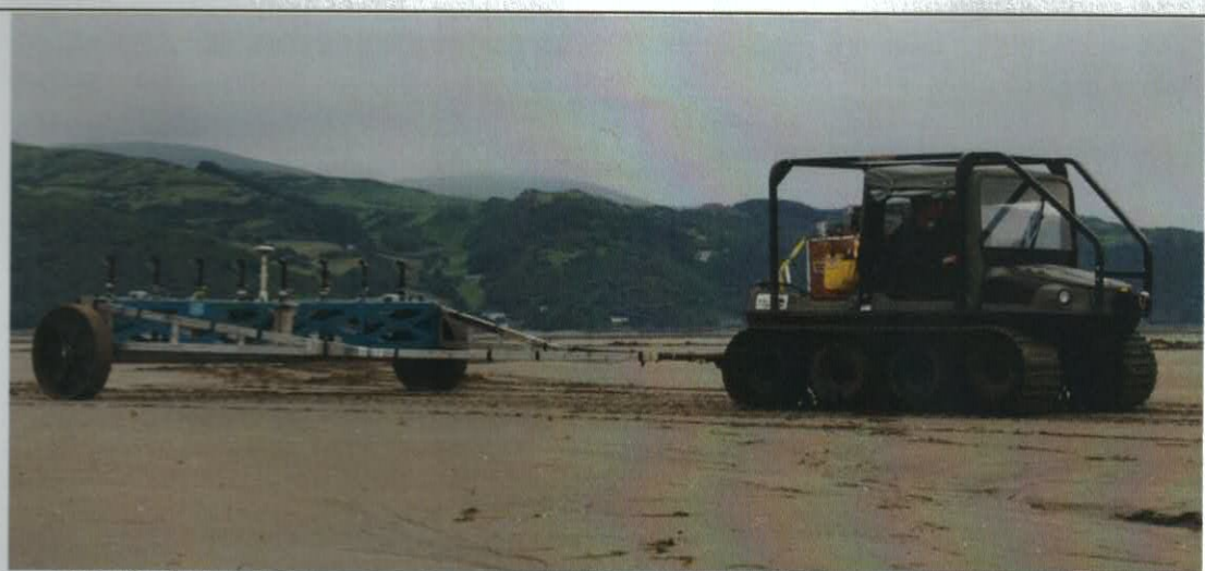
Plate 2: 4m array fitted with 8 probes towed by a tracked Argocat within the Dyfi estuary.
