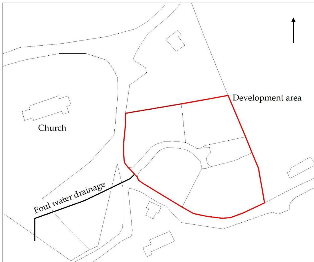
Fig. 3: Development area layout showing route of foul water drainage.
