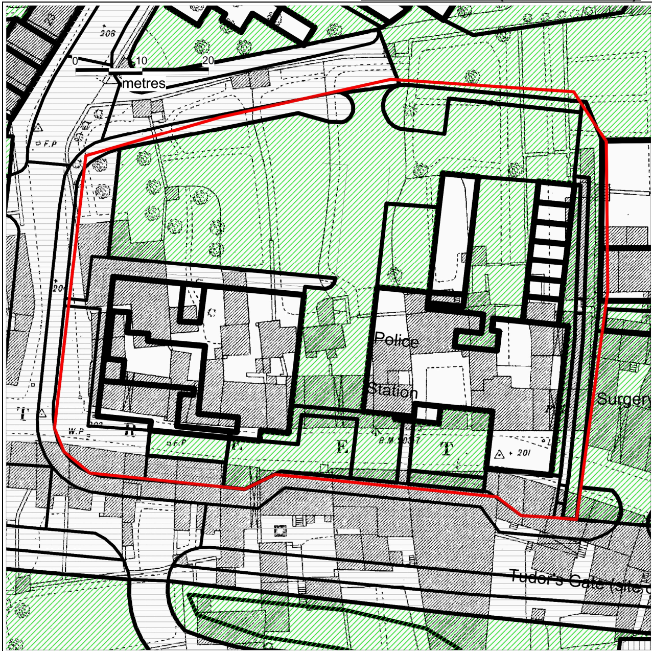
Figure 1; The 1881 1:500 Ordnance Survey map overlain by modern Ordnance Survey mapping. The approximate development area is outlined in red . This shows that the old road line ran slightly north of the present road and also that a number of the buildings demolished in 1958 stood beneath the Magistrates Court and Police Station, within the proposed development site.
