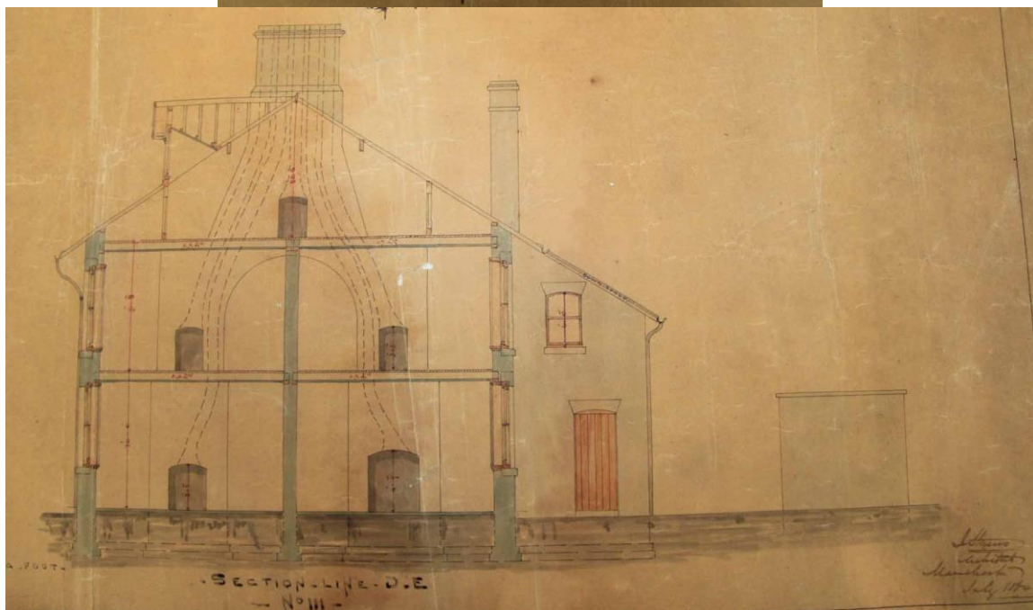
Fig 5 Cross-sections of proposed houses, showing one with transverse stair (13-18 Heol y Dwr / Water Street) and one with an attic storey and overhanging eaves (19-24 Heol y Dwr / Water Street), drawn by James Stevens of Manchester. (© Talyllyn Railway Archives)
