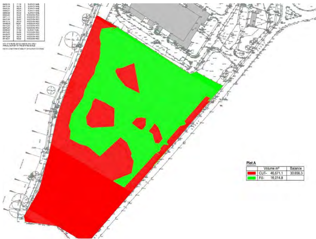
Figure 7: Schematic plan of cut (red) and fill (green) proposals for the development site.
