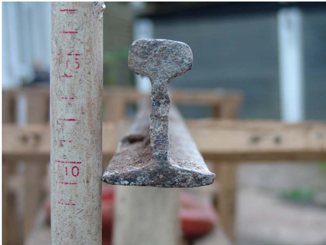
Plate 15: Profile view of steel rail. Scale with 0.2m increments
