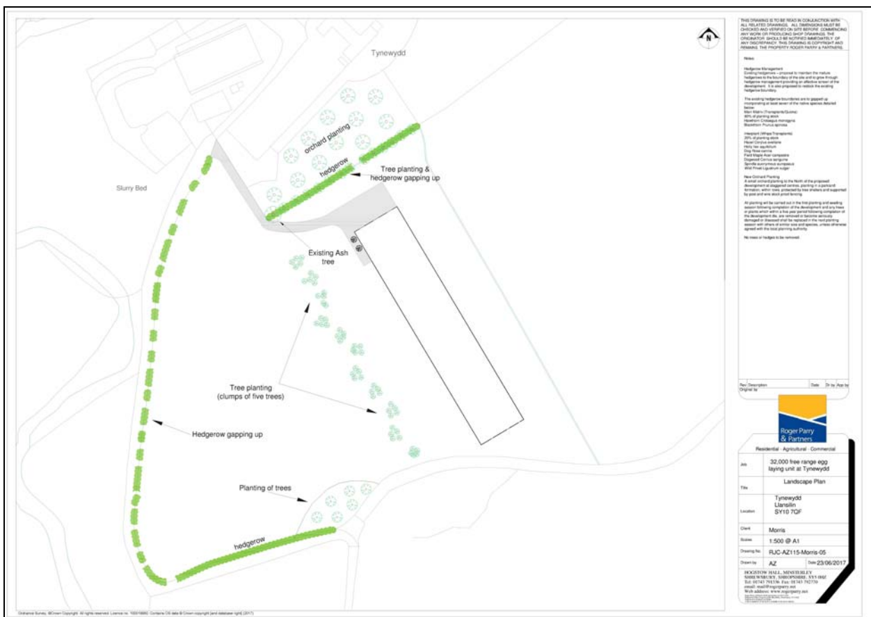
Figure 2: A plan of the proposed development, illustrating the position of new tree planting which will screen views of the building from the south and southwest.
