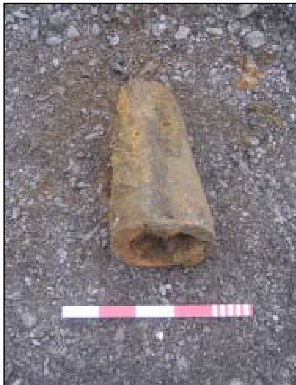
Plate 47 The 19th century cast iron tuyere that was recovered from the site of the 'new puddling' (forge)
