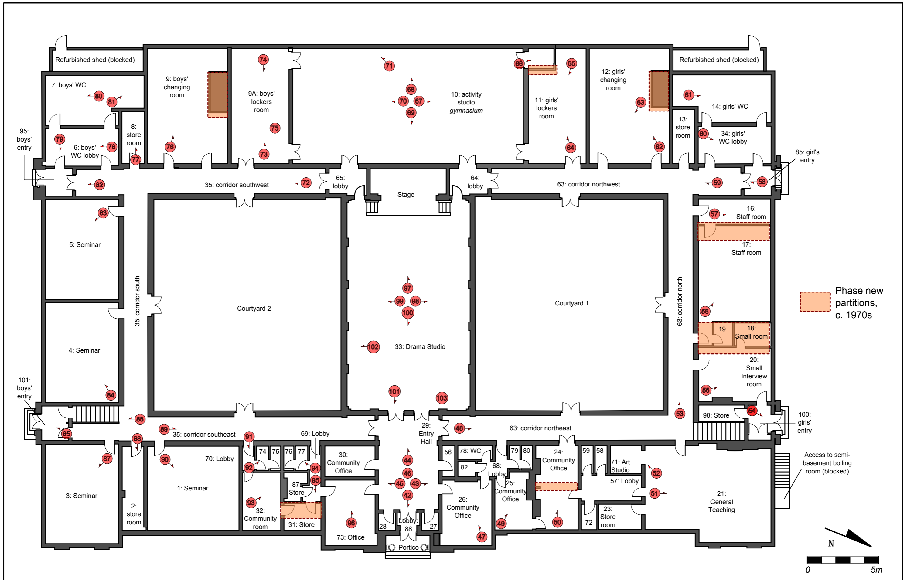
Figure 11: Plan existing rooms within the ground floor and new partitions, with plate numbers and direction of shots.
