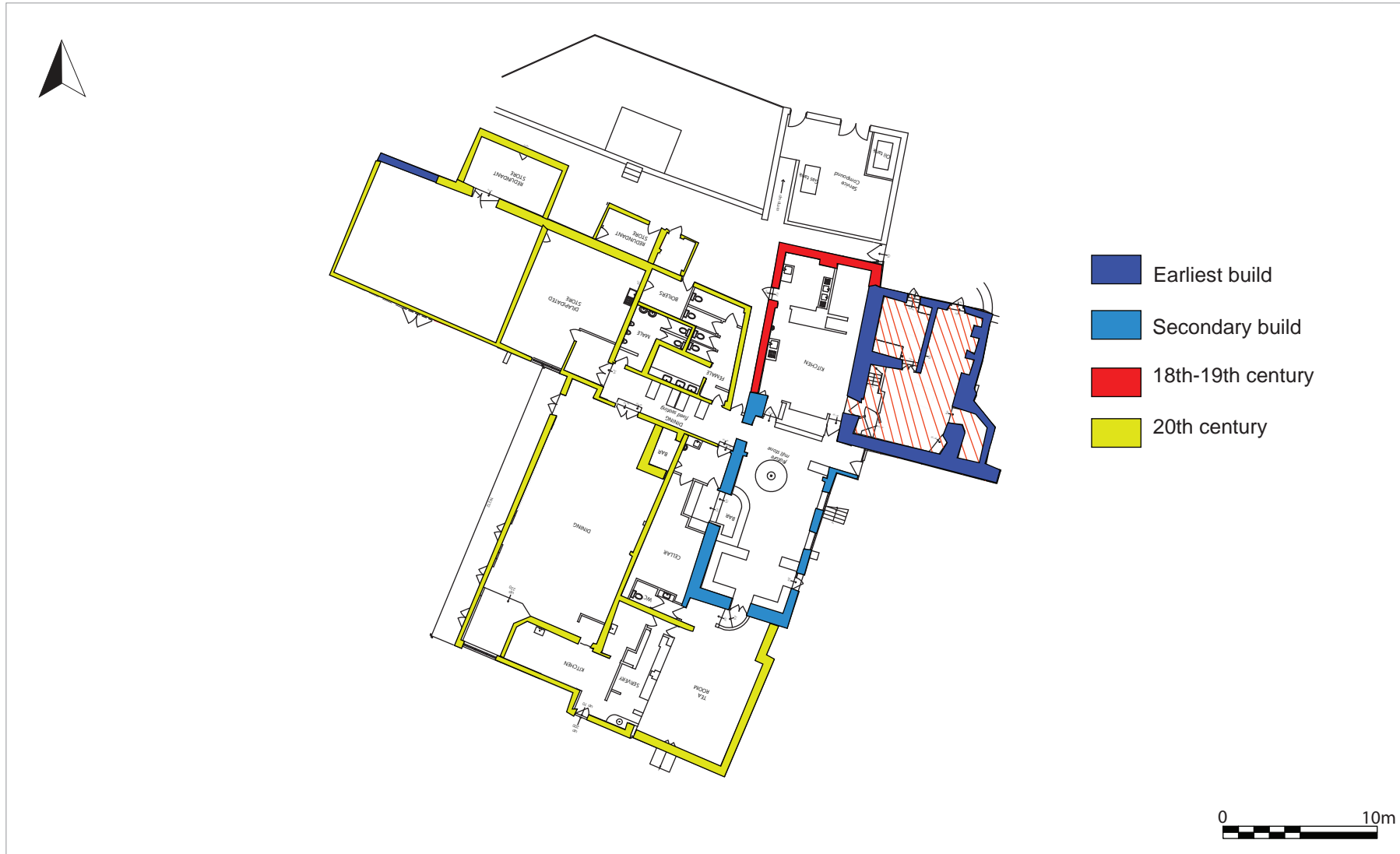
Fig 4: Structural phasing of the Anchor Inn, Tintern (After ADS Design groundplan)
