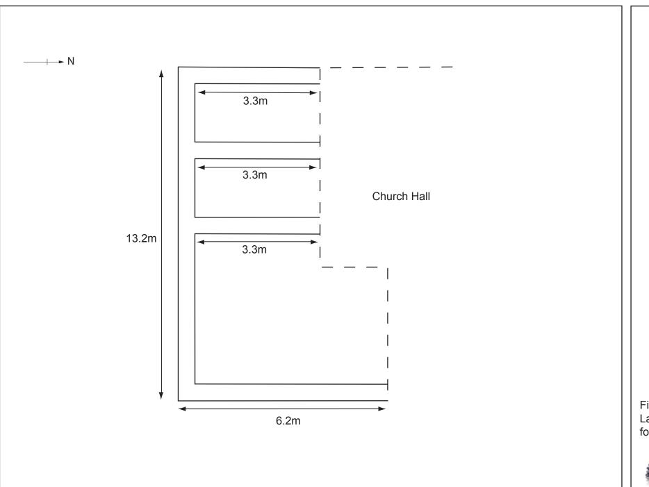
Fig. 2 Layout of footings trenches
