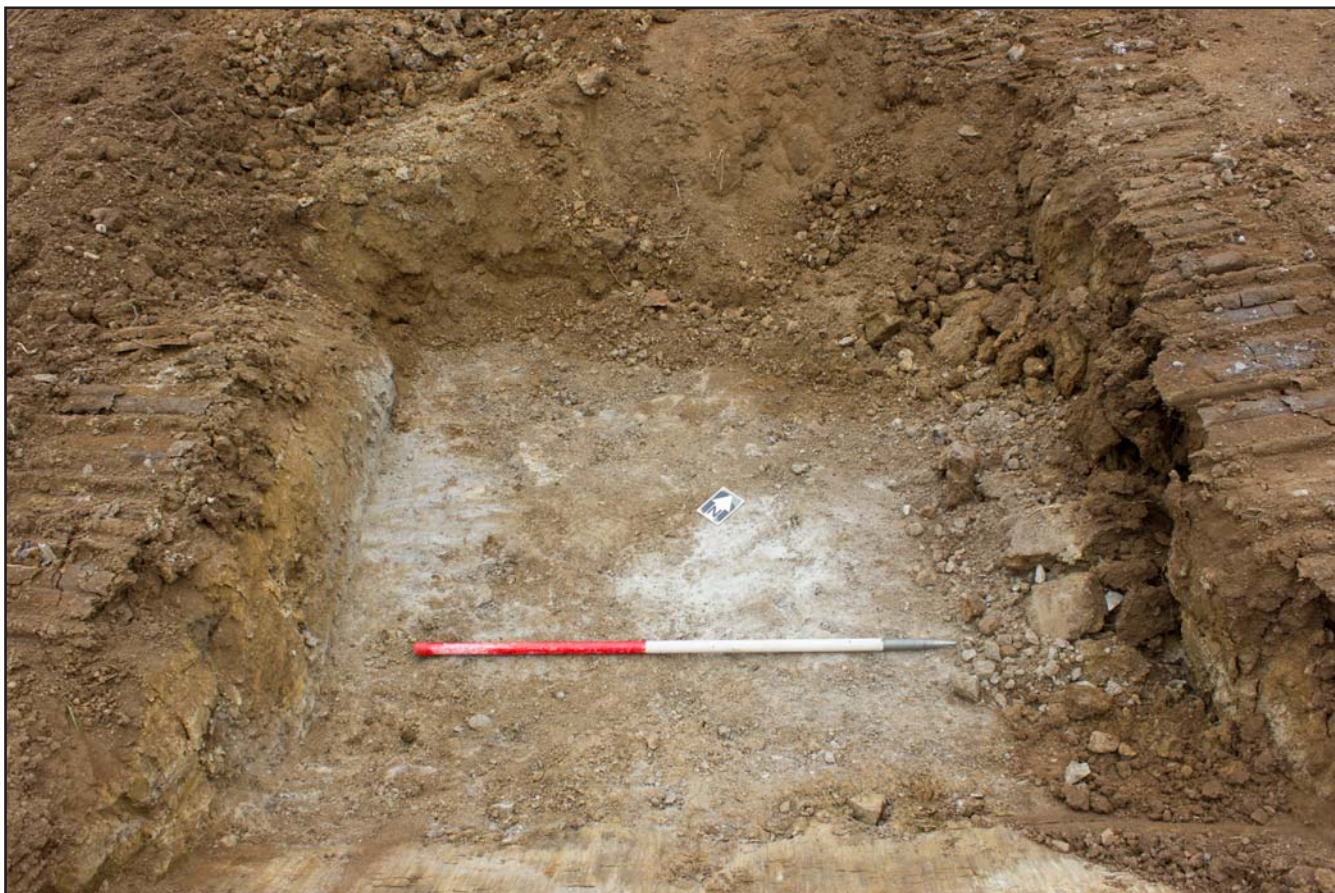
Plate 07: CBR Pit 2 in Plan (CH70), Parc Bryn Cefni, Llangefni, Ynys Môn - from the southeast - scale 1m
