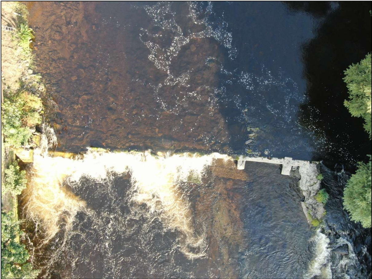
Fig. 7 Overhead drone survey photograph of the weir (west is to the top of the photograph). Note the line of a possible earlier structure upstream of the extant weir (left of shot).
