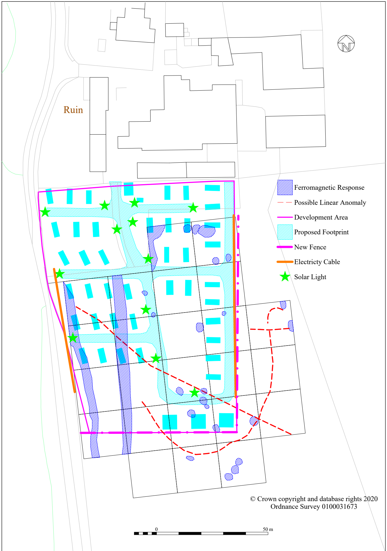
Figure 9: Correspondence between the Proposed Development and the Survey Results Scale 1:1,000
