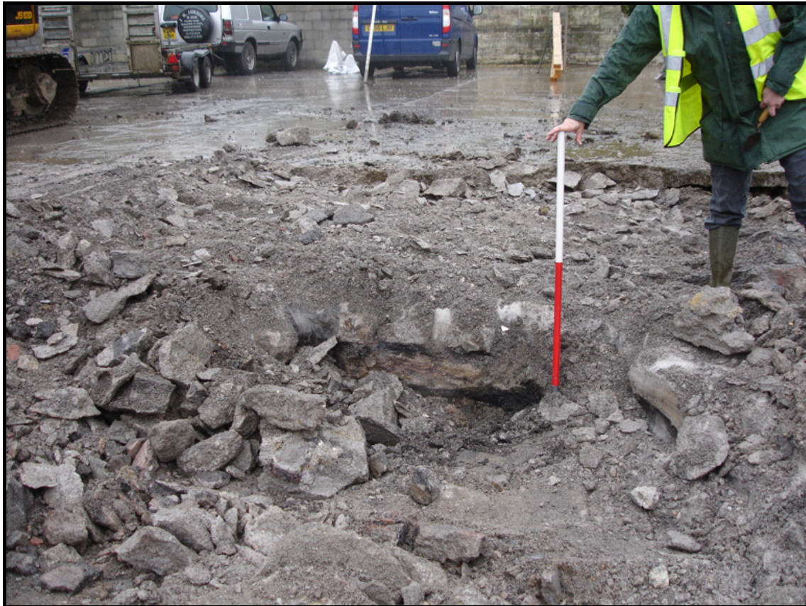
Plate 3: CYG003 - Partial section of Pit 1 showing the capping concrete, context 001, and the loose layer below, context 002
