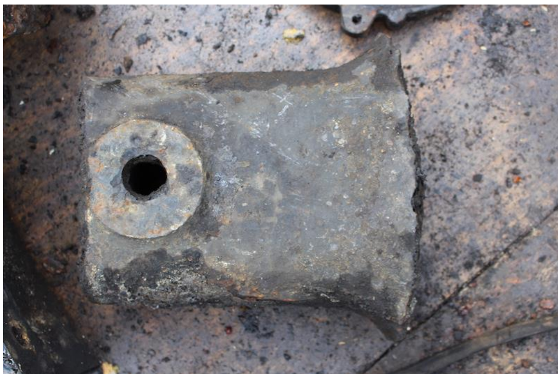
Plate 78. Very large cast counterweight recovered from wheel pit [206].
