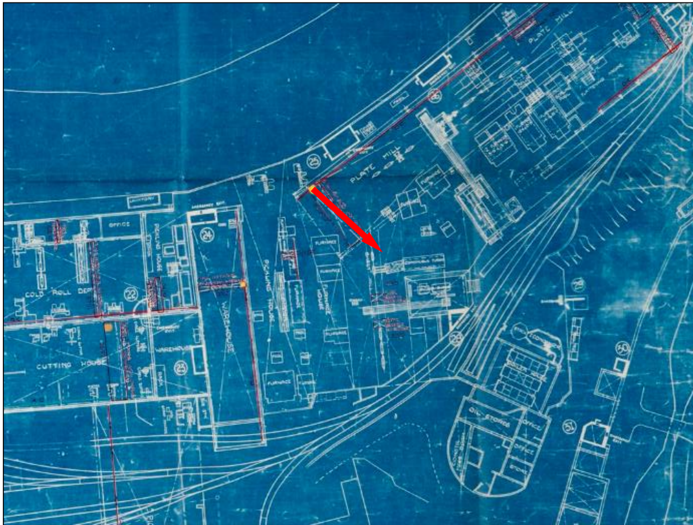
Figure 5. 1939 ICI plan of Hafod Copperworks showing the Vivian Engine House. The Vivian Engine House rolling mills appear to be fitted with electric drives. Note the additional rolling mill drive just above the Vivian Engine House in this plan. © National Museum Wales
