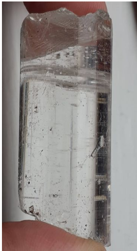
D11 , left: fragment of cylindrical/rod glass insulator, precise function unknown. 24mm OD.
