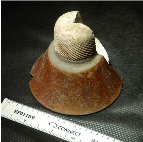
C25 , above: Part of the P.5656, nested insulator with a central threaded section containing cementing and a lead (metal) collar.
