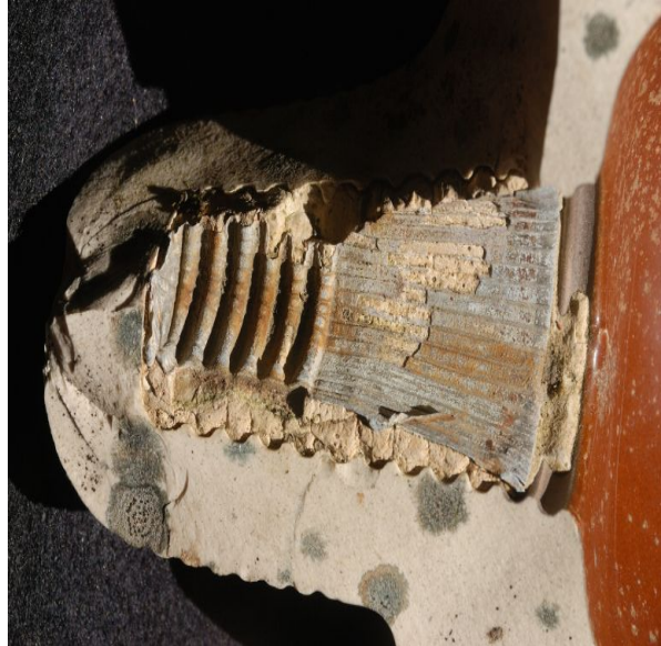
C25 , above: Part of the P.5656, nested insulator with a central threaded section containing cementing and a lead (metal) collar.
