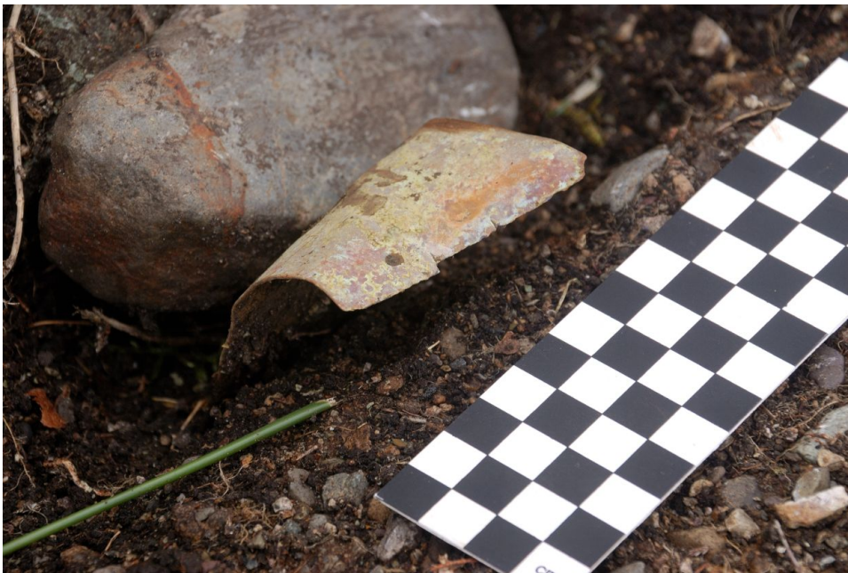
Stay cable anchor block 13/17A grounding strap, cut by salvagers at the centre rear of the anchor but with 95cm of the strap remaining in the ground. Scale squares = 1cm, not indicating north.
