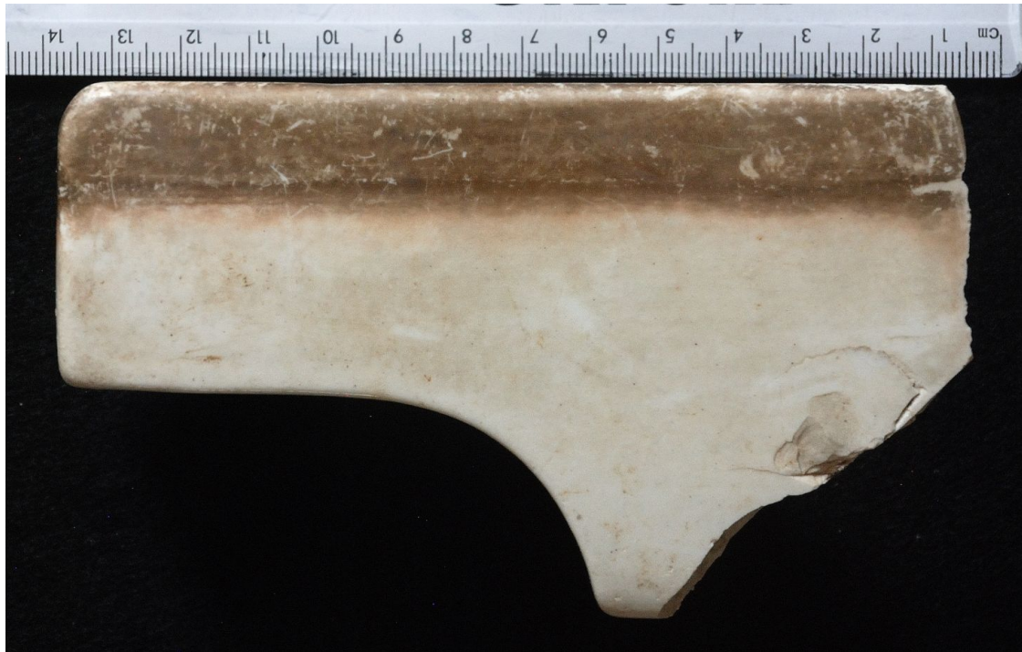
C19. Side view of one end of the insulator. No maker's impression has been found on any fragment to date. Scaling from images to fragments allowed the intact length of these insulators to be determined as ~2 feet at the top, ~16" at the bottom.
