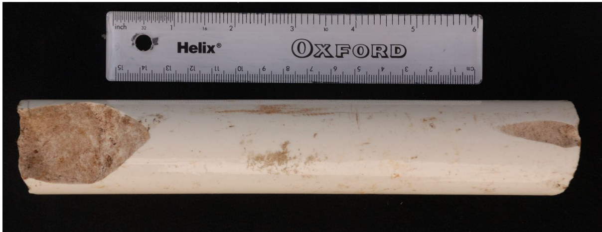
28. Ceramic rod insulator fragment recovered at Carnarvon. These were used extensively for various purposes around the site. Scale = 150mm/6"
