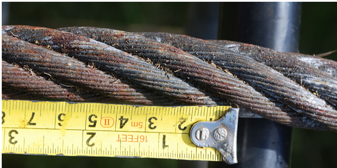
19. 1" diameter stranded stay cable – usually then termed 3" [circumference] cable – was discovered, buried at the western foot of the octagonal concrete base (see 108 ) during fieldwork. for this study.
