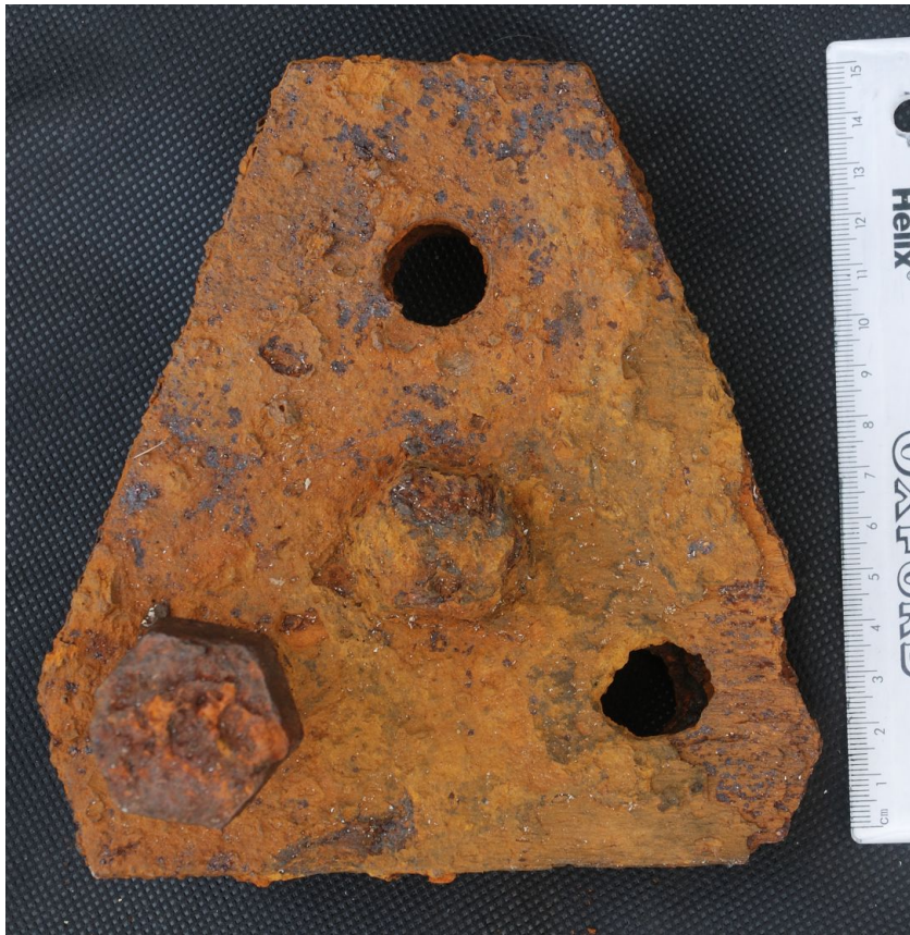
134. An anchor-to-two-stay attachment plate. The top hole bolted to the loop on the anchor, the lower holes, one with a bolt still in position, each attached a stay wire. This was found near the wall and below blockhouse 5 on the upper part of the 1923 extension site. It may have been one of the main anchor attachment plates. Found as bolt surface protrusion, at 53.122857°, -4.173596°.
