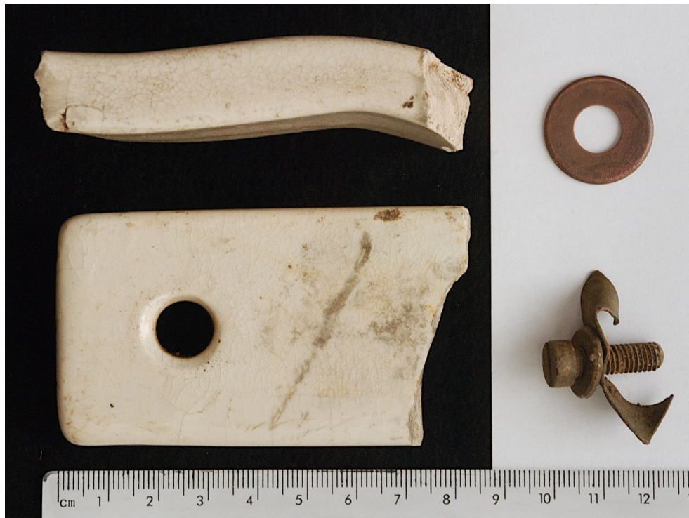
C14, left. Ceramic fragments from the upper ATI house. Their function is not yet determined. Right: copper washer from upper ATI house, and slotted-head bolt with washer and copper earthing strap from the lower ATI house.
