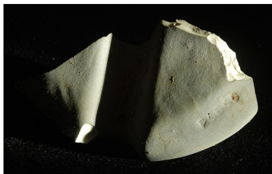
C27 , right: top element fragment of the same insulator, bearing the P.5656 part number. Little of the original brown glaze remains.
