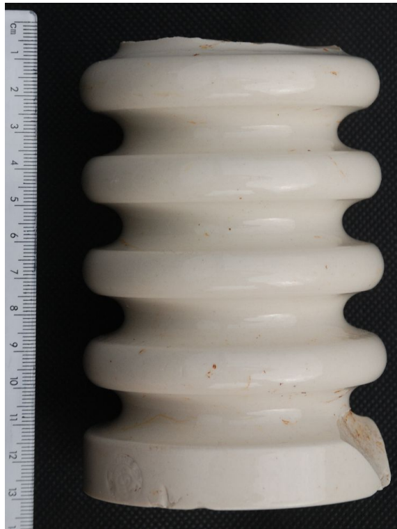
C23. Cylindrical ribbed insulator, bearing Taylor and Tunnichiff impression (at lower left), found at the double inductor house. These had many uses, similar ones seen in use at C19 .
