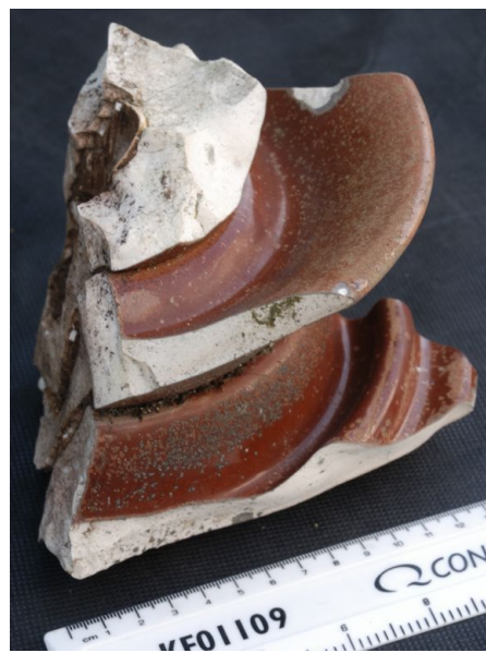
C26, a and b , below: some of the components still cemented together in a separate discovery. It is not known for certain for which element of the antenna or earth system the insulators were used.
