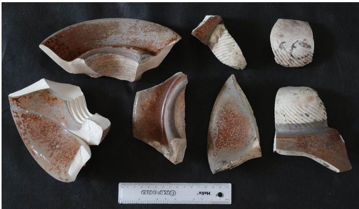
C24. Fragments, at least two pieces from the same insulator, where the outer brown glaze has severely deteriorated. These were parts of a nested insulator, cemented together, and found close to a counterpoise lattice mast, upon which it is thought most likely was mounted. The larger fragment at far right has a maker's number, P.5656 (see detail, below). The top centre fragment has the same, but partial P.56...mark. A single top piece (not shown) bearing the same P.5656, has a groove of ca. 15mm diameter for receiving a wire, which may add to the belief this was a counterpoise masthead insulator, though the groove may not have been used.
