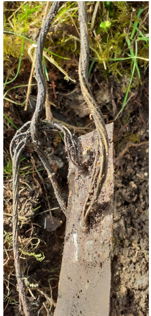
Right: detail of two, 7-strand copper wire metallurgically bonded to the copper grounding strap. The bonding remains strong and mostly uncorroded after 100 years in the ground.
