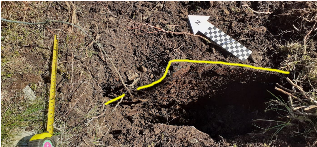
D13 , below: detail of wire connection to plate, the upper plate edge highlighted in yellow line. Tape open to 1ft, north indicator scale in cm squares.
