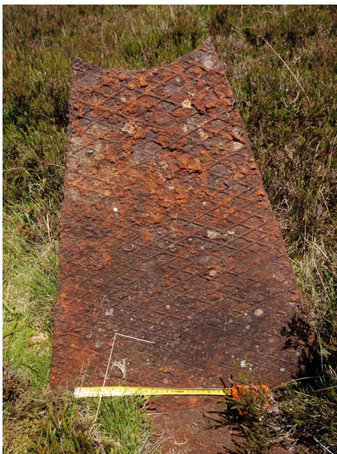
5. Tread steel plate, with inner and outer curved edges, possibly part of the standing area of a mast-top gallery, potentially Mast 8, which is seen in a 1939 British Pathé film reel ('Felling Wireless Masts at Carnarvon', Film ID: 1013.05, issued 1/06/1939) to fold on toppling, which might explain this plate being found 265', and not 400' from the mast base. Yellow part of tape open to 1 foot. 25¾" long, outer edge 21¾" long, inner edge 9½" long, ½" thick.
