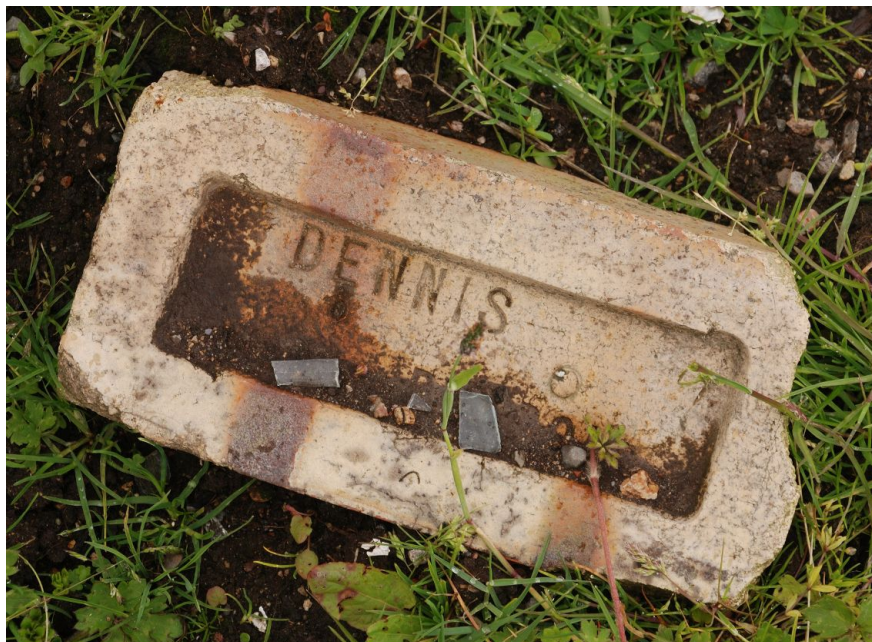
C32. Brick made by Henry Dennis at the Hafod Brickworks, Ruabon (active from ca. 1867). Dennis bricks were claimed to be amongst the best quality and most widely-used bricks in Britain at the time. 'Ruabon' impression mostly obscured at bottom right of central 'frog' indentation.
