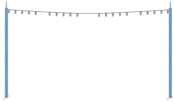
14. General arrangement of 1914 mast heads, triatic support wire widthwise between them and insulator supports hung from it. The lower insulators were 'reel' (pulley-wheel) type, through which the antenna wire moved freely to allow for dynamic tensioning from the rear, where triatics had a design breaking strain of 7\frac{1}{2} tons (draft specifications appearing in The Marconigraph , September 1912, pp. 214-216). The view is looking either up or down hill, along the antenna. This depiction, for clarity, shows just 20 radiating wires, whereas there were 32 initially. Two wider gaps between sets of insulators are inferred from the pattern of the rear wire strainers and the centre gap inferred due to the presence of central towers at either end of the array.
