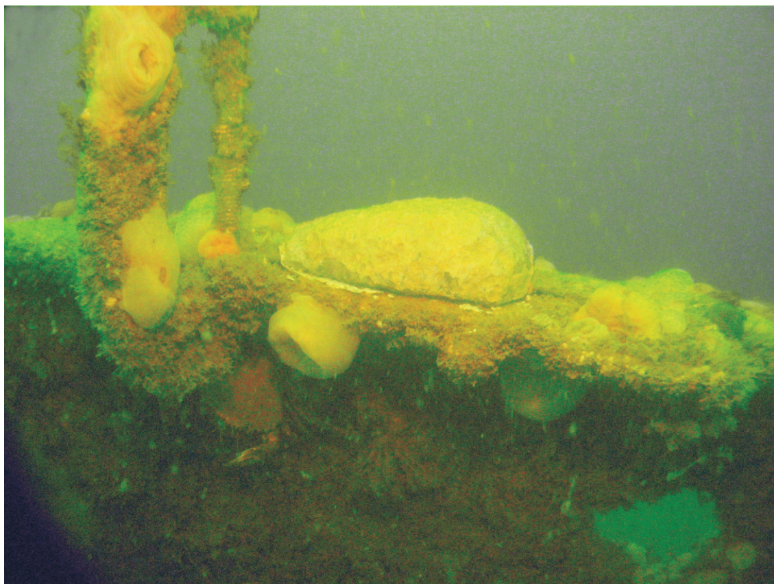
Plate 3. Anodes on top of conning tower
