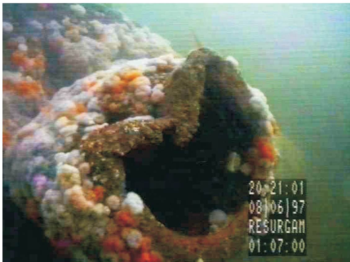
Plate 4. Damage to conning tower, 1997 SubMap photograph
