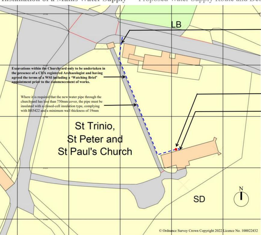
Point of entry for the new mains water supply from the Highway approximately 1200mm away from the boundary with the adjacent property. Incoming water supply to be installed in accordance with the standard utility providers details.
