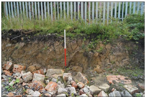
Plate 15: A view of a thin dark peaty soil overlaying boulder clay exposed to the southeast of the lamp room building. Looking southeast.
