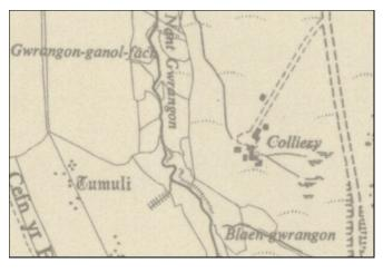
Figure 7; The Ordnance Survey 1:25000 map of 1954 (Sheet SN90 – B) is the first to show the No.4 shaft of Tower Colliery. The survey was undertaken before 1950 when the mine was relatively new and shows the complex to include the pithead building, engine house and lamp room and office building. The pithead baths building had not yet been added.
