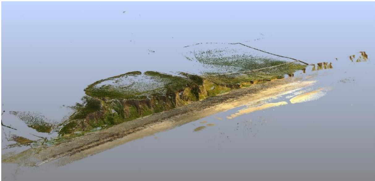
Figure 6: Raw point cloud of the cliff face derived from laser scanning survey (© Crown copyright: CHERISH project 2018).
