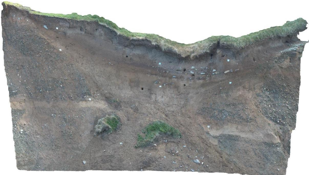
Figure 13: Orthomosaic of the southern ditch section created from overlapping SfM UAV imagery in Agisoft Metashape. Ground Control Points(white targets) were used to georectify and scale the image. The series of layers within the ditch can be seen along with the circular holes where OSL samples were taken. Crown Copyright: CHERISH Project
