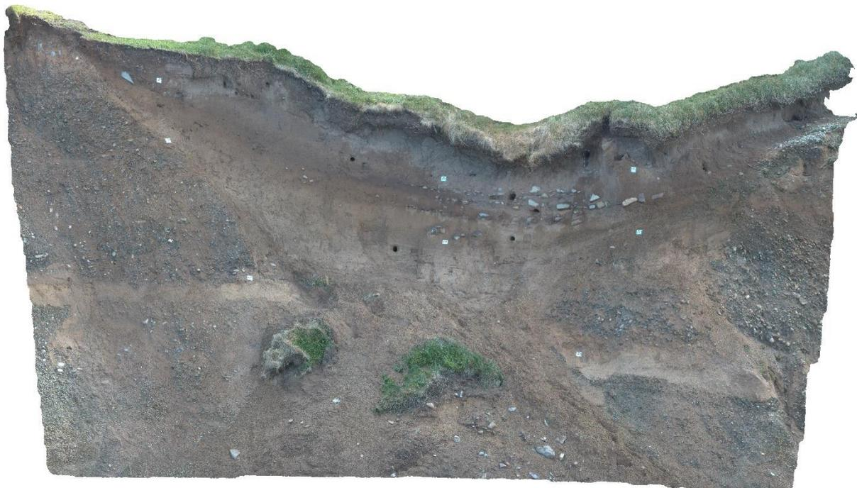
Figure7: Orthomosaic of the southern ditch section created from overlapping SfM UAV imagery in Agisoft Metashape. Ground Control Points (white targets) were used to georectify and scale the image. The series
