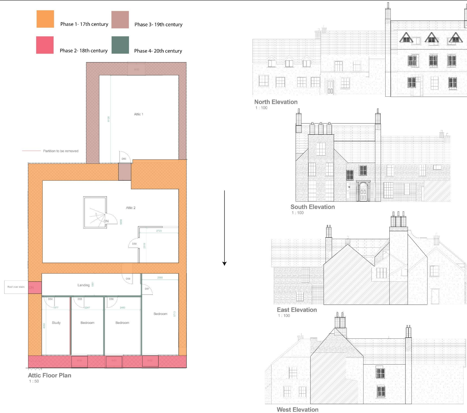
Fig. 30 Second floor plan showing construction phases (left) and position of original house in relation to existing structure (right)
