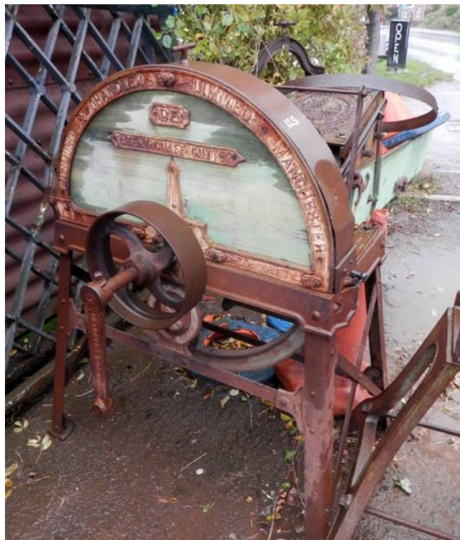
Fig. 16 Richmond & Chandler chaff cutting machine (Grace's Guide Im20121018)
