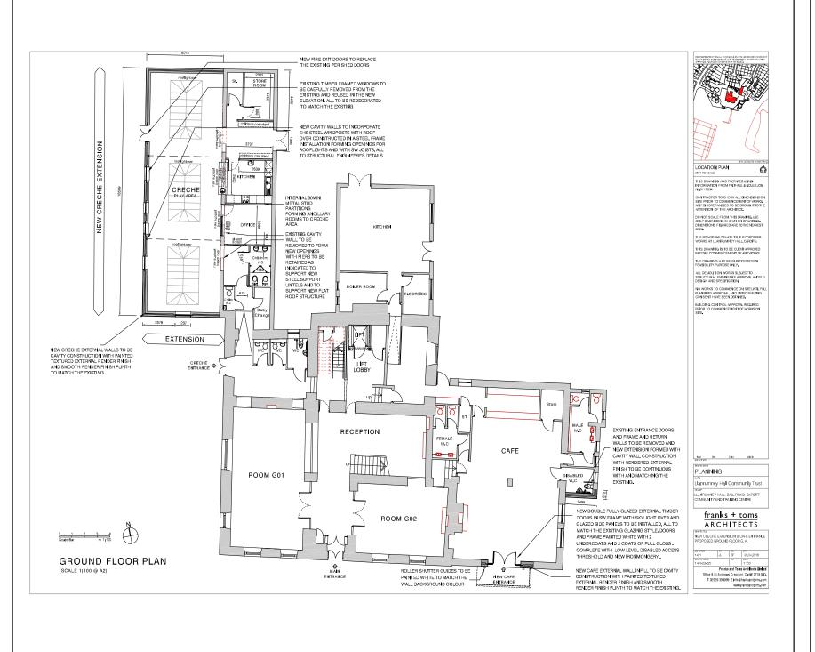
Figure 2. Proposed ground floor plan showing the new extension in the top left corner.
