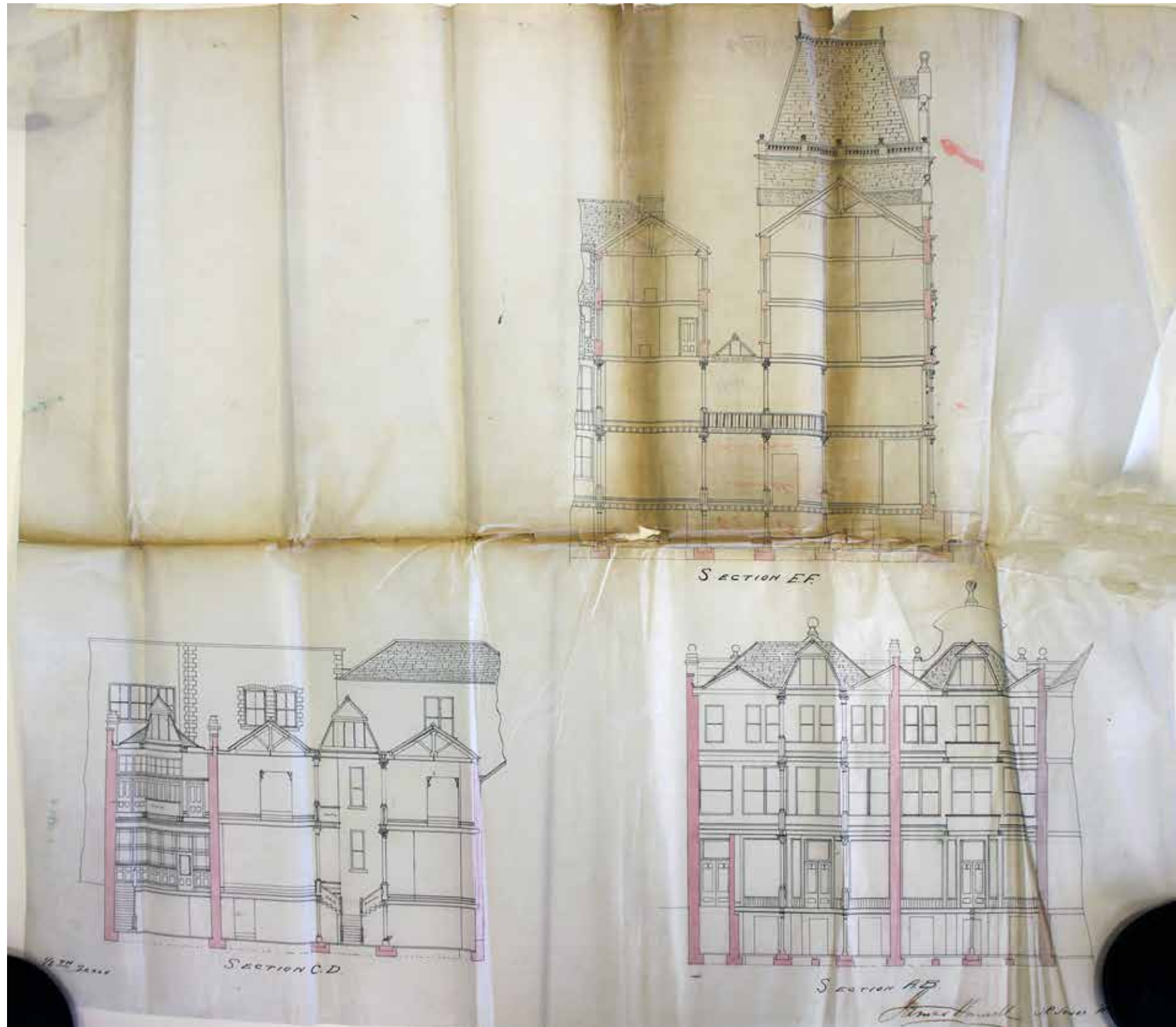
Sections through the Trinity and St Mary Street buildings produced by J.P. Jones in 1888 showing the Trinity and St Mary Street buildings. Jones's 1888 additions are tinted in pink. Section E-F cuts through the northern part of the 4/5 storey St Mary Street building. Section C-D shows the the eastern portion of the St Mary Street shop floor, Section A-B shows the inner face of the Trinity Street façade. (Glamorgan Archives)
