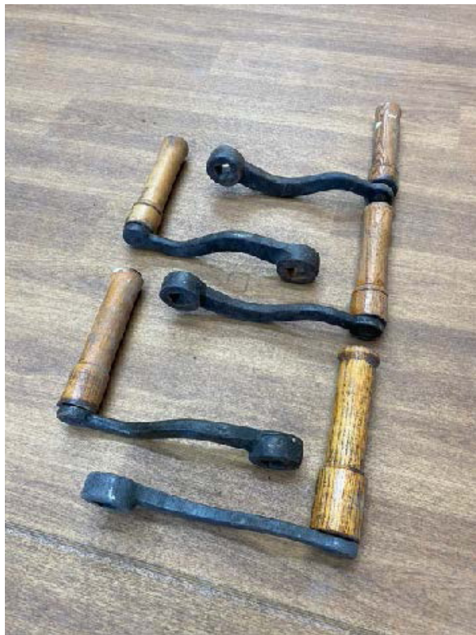
The four wrought iron and hardwood rotary handles found within the Market Hall.
