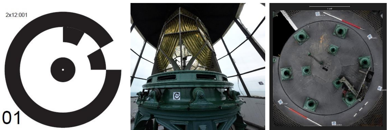
Figure 2.2. Photogrammetry targets used to aid image alignment. Left: Example target. Centre: Target in-situ on pedestal and lantern window. Right: Orthomosaic plan of targets and scales on the lantern room floor (@ Crown Copyright: RCAHMW).
