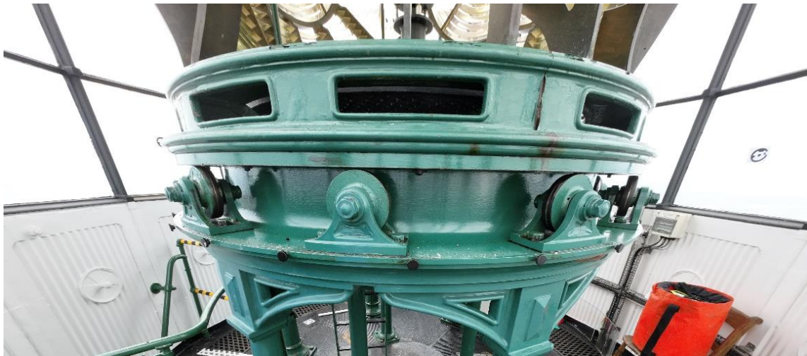
Figure 4.6: Support wheels around the outer upper-band of the pedestal. The turntable gently rests on the support wheels (© Crown Copyright: RCAHMW).
