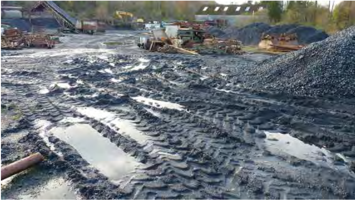
Photo 5: View showing typical ground conditions across the site, consisting of coal sand overlying hard-core rubble.
