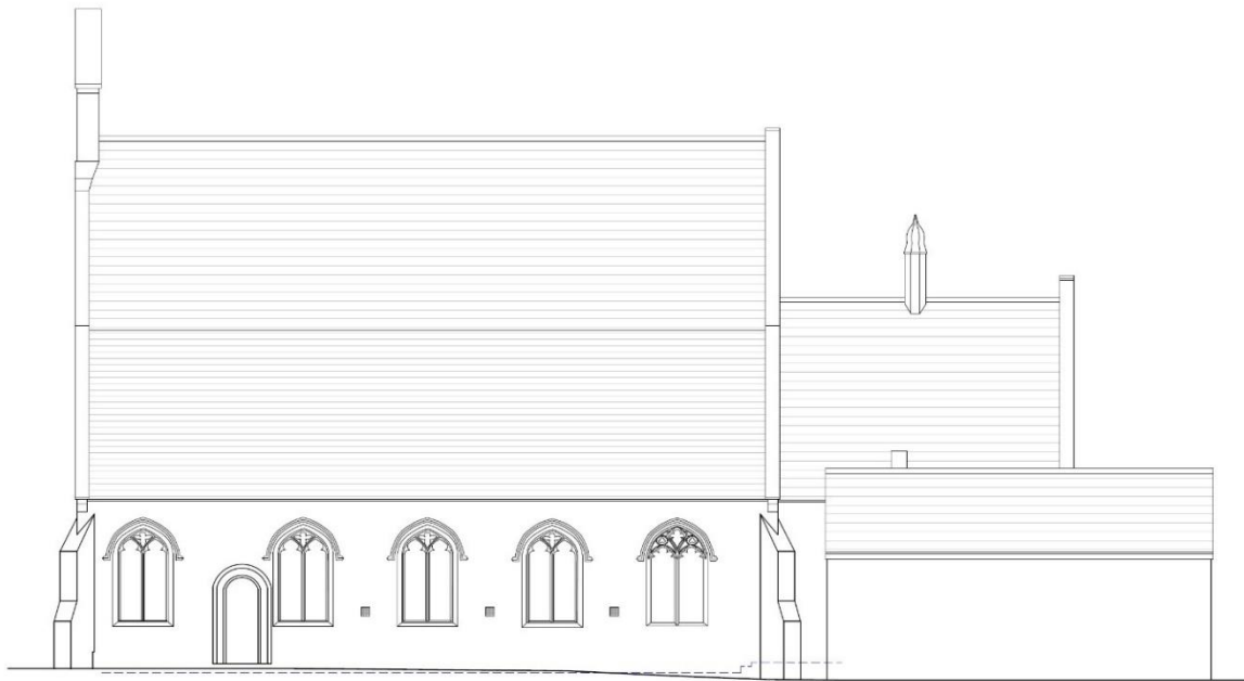
Figure 8. Elevation showing the south aisle and vestry.
