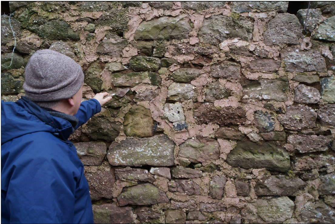
Plate 56: GTB2021_056 - A view showing Martin Locock taking Mortar Sample E from the eastern gable wall of the threshing barn. Looking east-southeast
