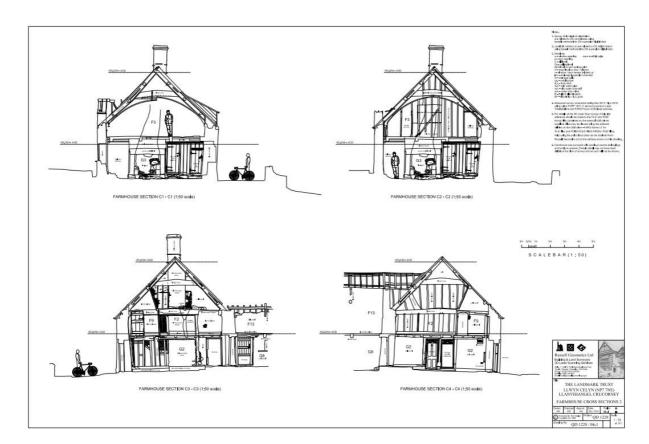
Fig.16: Cross-sections of the main House.
