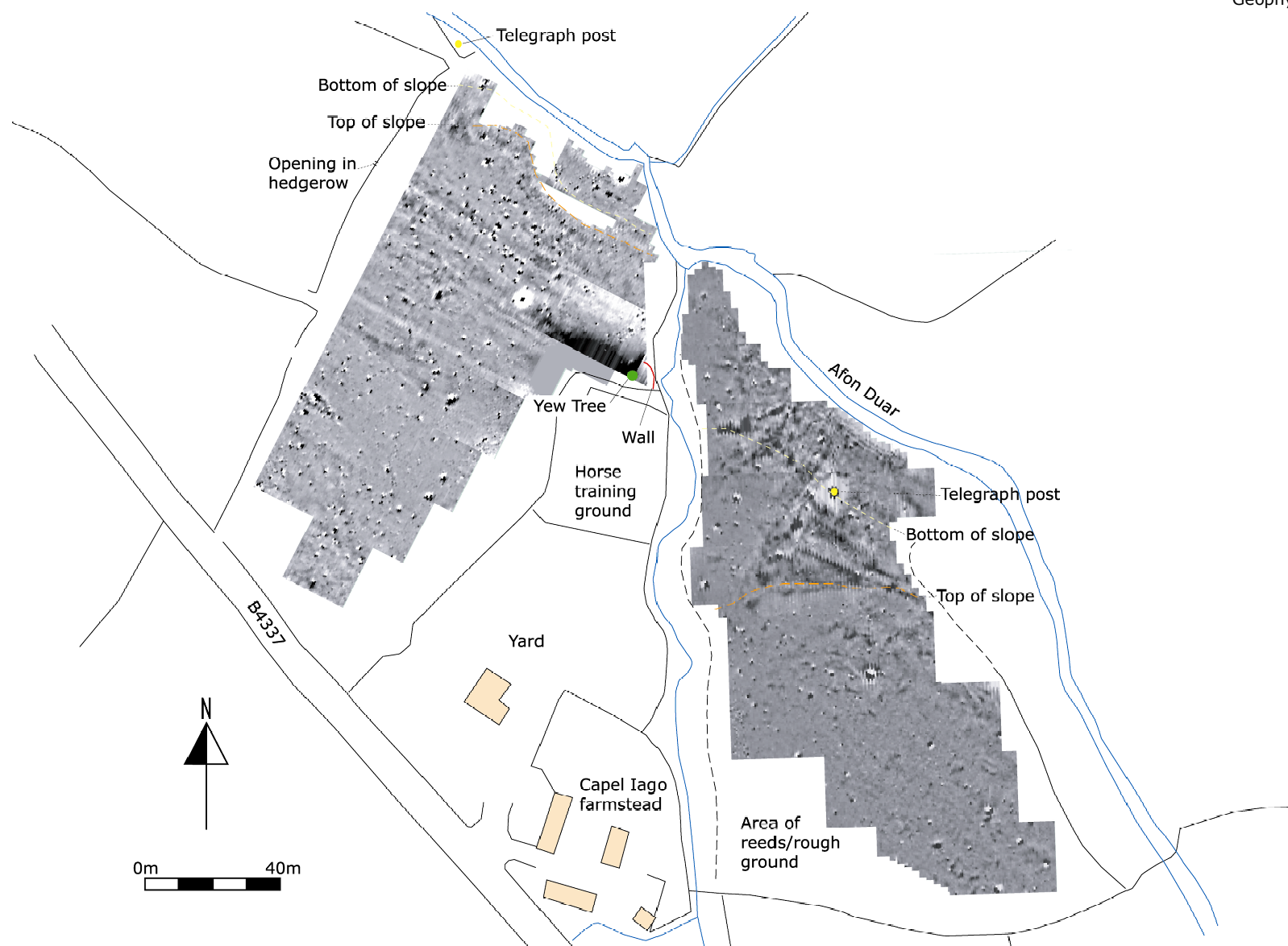
Figure 6: Geophysical survey results presented as grey-scale plots, overlaid on local topographical features
